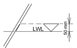
The height of the triangle in the **vertical plane** shall be not more than 50mm
