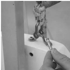
Attach the short lifting slings to the aft holes on the inner chainplates and the long slings to the fittings on the upper gudgeons.
