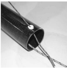
The spinnaker halyard will be passed through the pole launcher line block in order to extend the pole when hoisting. As the block is pulled up into the bow under the cowling when the pole is retracted, it is important to reeve a "mouse" line through the block to enable you to easily reeve the spinnaker halyard after you have stepped the mast.
