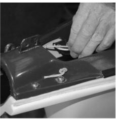
Pass a "mouse" line through the sock to assist when reeving the spinnaker halyard. Attach without tension both fore and aft. Tie the gennaker sock to the saddle fitted on the aft bulkhead.
