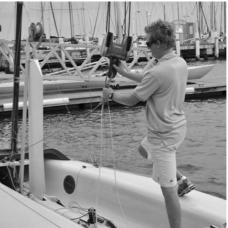
After disconnecting the lifting slings, carefully lower the centreboard with the manual winch, then remove the keel lifter. Insert the lock-down pin.
