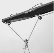
Pass forward through the block located above the cleat, down to the ratchet block and through the cleat.
