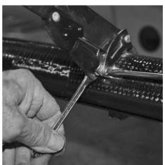
Fit the shrouds to the mast with the t-bar terminals by inserting and rotating the terminal 90°. Position the shroud wire in forward section of the spreader tip clamp.
