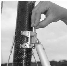
Use the cleat on top of the boom to set "topping lift". Attach compression vang line to vang tackle hook block
