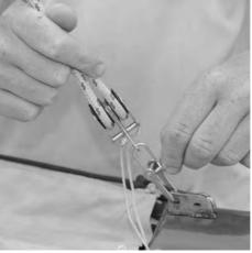
Haul down on the rig tensioner until the forestay pin can be inserted, then cleat off. Secure forestay pin with split pin or snail clip. Uncleat rig tensioner and slowly release load on to forestay. Remove rig tensioner.
