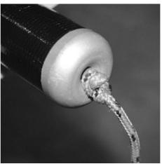
With the pole fully extended and all slack taken out of the line, tie the inboard end of the tack line off to the shackle at the front of the aluminium rack in the centre of the boat. This limits the pole extension.
