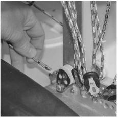
Once hoisted, the jib halyard tension is controlled by a separate hauling line attached to a cleat that is fitted to the halyard above the deck.
