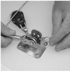
Place some cushioning on the floor of the cockpit to prevent damage when raising the mast to vertical by pushing against the step.
