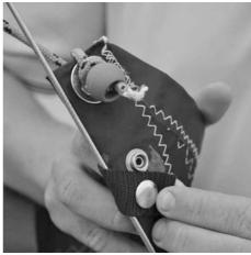
Shackle the tack eye on to the aft hole in the stemhead fitting. Wrap the jib luff pocket around the forestay and zip closed to hide the wire strop and eye.
