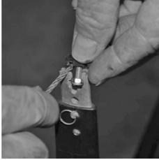
Remove the slack in the wire from the upper terminal and tighten the clamp. Repeat for the other side. Use the slide adjusters on the spreader tips and turn the barrel adjusters until wire to wire measurement is approximately 770mm and distance from aft face of mast to the transverse of the shrouds is approximately 190mm.
