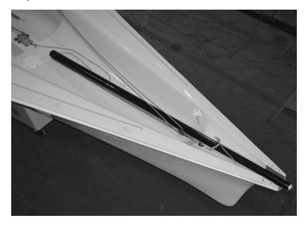
Place the pole into the groove in the bow. Make a lashing that is tight on the pole when it is extended until the inboard end of the pole is approximately 10cm from the lashing. Feed the gennaker tack line through the hole in the tip casting, through the pole and into the boat, and tie a figure 8 stopper knot leaving approximately 30cm of line to attach the tack.
