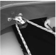
The halyard is led back to the turning block mounted on the aft cockpit bulkhead near the floor and from there into the gennaker sock. Use the mouse line to haul the gennaker halyard forward through the sock until it exits at the bow.
