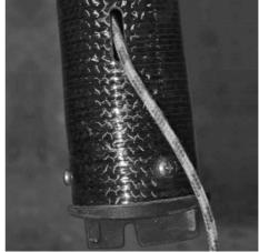
For an external system, the halyard is passed through the spreader fitting (it may be necessary to grind off some of the inboard end of the port spreader arm) and directly through the deck eye in the cowling.
