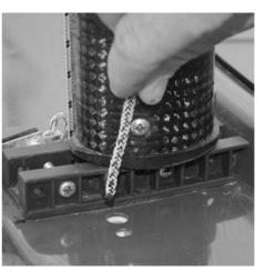
The halyard is led through the cowling and to the turning block at the base of the mast post to provide an ergonomic point from which to haul the sail aloft. Tie a stopper knot in the end of the main halyard once reeved.
