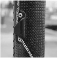
Attach the outhaul line that feeds through the port side hanging block on the inboard end of the boom to the outhaul tackle. Ensuring the compression vang is also attached to its tackle, wrap the mainsail luff pocket around the mast.
