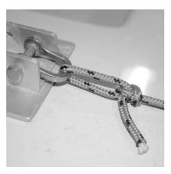
Pass the end of the pole launcher line (with the block attached) inboard through the bow turning block, then through the grommet on the inboard end of the pole and tie a stopper knot that will pull up on the inside of the pole. Ensure there is a small amount of slack in the pole launcher line when the pole is fully retracted.
