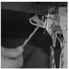
Use the mouse line to reeve the halyard end through the gennaker pole launcher block and back aft (above the sock and pole but below the jib sheets) between the cowling and the cleat console platter and through the spinnaker halyard deadeye and cleat.
