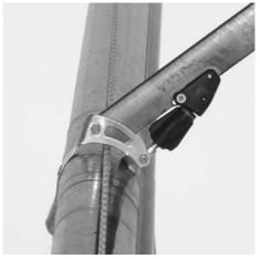
The main halyard is a 2:1 system dead-ended at the masthead fitting and reeved inside the mast and exiting on the starboard side near the foot.
