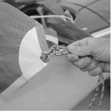
Untie the retrieval end of the halyard from the mouse line and tie a bowline through the eyelets in the gennaker retrieval patch, making sure this section of halyard runs clear from the throat to retrieval patch. Tie both ends of the gennaker sheet to the clew of the gennaker using bowlines.
