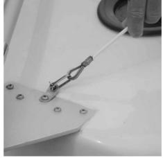
Attach to the crane hook and raise the boat taking care to avoid contact between the mast or spreaders and the crane jib. The aft slings may be adjusted in length to provide a slightly bow down attitude. Ensure the boat is controlled by a tag line when using a crane.
