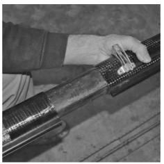
Fit the spreader arms and adjusters using the supplied bolts & nyloc nuts. Note that the adjusters are coded red and green for port and starboard.
