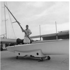
Lift mast and place in mast step. One person remains holding the mast forward, while another attaches the rig tensioner to the aft hole of the stemhead fitting or to the towing ring .
