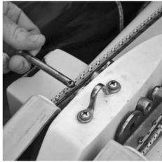
Fit the snail clip to secure the keel lock-down pin. Fit keel wedge (if supplied) and tap down behind the trailing edge until firm.
