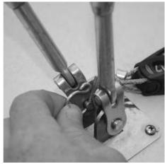
Adjust shroud tension to suit the sailing conditions.
