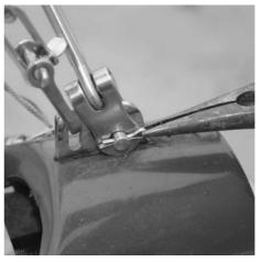
Attach the inner shrouds using the t-ball fittings and attach to the forward hole on the chainplates drilled with two holes.
