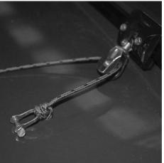
The secondary jib sheet is dead-ended with a stopper knot on the aft face of the cowling, passes through the deck eye, through the floating block and is cleated on the console.
