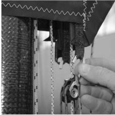
Pass the clew strap under the boom and clip on to the lower webbing loop, ensuring mainsheet is still free to travel. Attach the outhaul clip to the webbing loop on the clew.
