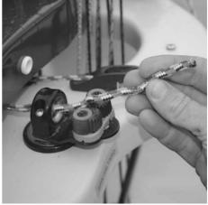
The halyard is then passed through the gennaker halyard tension block (attached to a length of bungee cord), forward to the turning block mounted on the port cockpit bulkhead or alternatively on the aft port face of the cowling.
