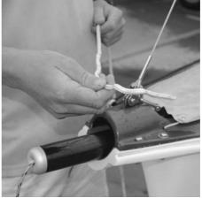
Taking the hoist end of the halyard and ensuring it runs clear from the hoist block to the port bow, tie a bowline on to the head of the gennaker. Attach the tack of the gennaker to the tack line using a bowline positioned as close as possible to the stopper knot.
